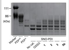
**Fig. 2**: Gel-band shift assay during the denitrosation of SNO-PDI.  $[GSH]^0$ =100  $\mu$ M,  $[Catalyst]^0$ =50  $\mu$ M, [PDI]=5  $\mu$ M at 30 °C, pH 7.5 for 60 min. PDI<sup>red</sup> and PDI<sup>ox</sup> mean reduced PDI and oxidized PDI, respectively.
